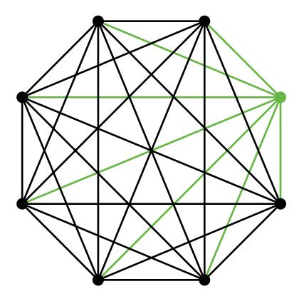
Iteratively add a new vertex connected to the vertices of an existing clique (complete subgraph).
