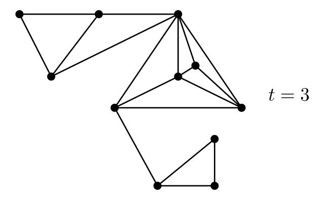
Iteratively add a new vertex connected to the vertices of an existing clique of size at most t.
