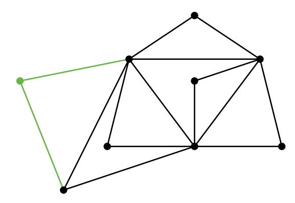
Iteratively add a new vertex connected to the vertices of an existing edge.
