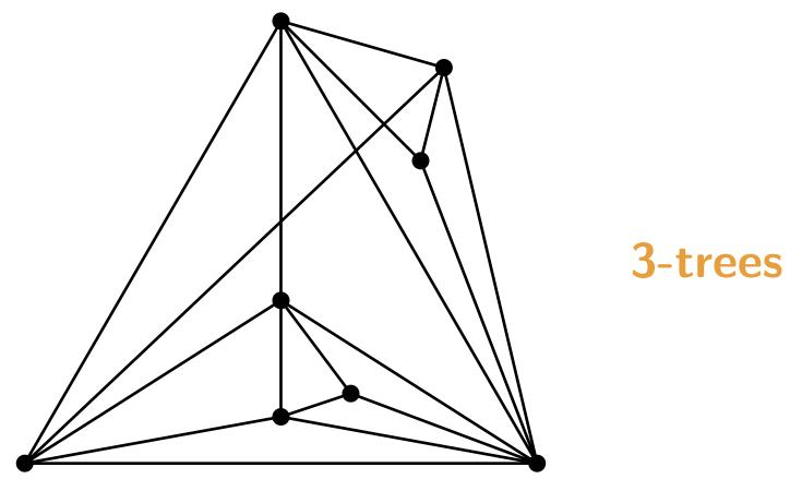
**Definition.** A *k*-tree is a graph obtained from a (k + 1)-clique by successively adding a new vertex connected to all vertices of an existing *k*-clique.
